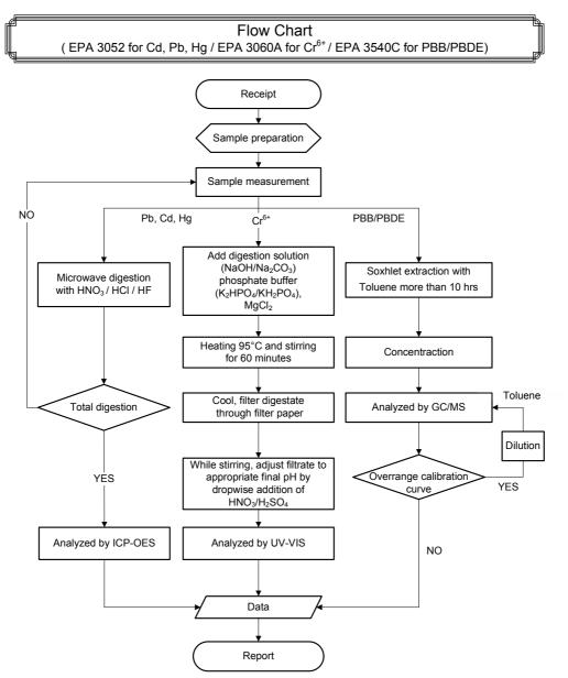
\*\* Remarks : The samples were dissolved totally by pre-conditioning method according to above flow chart.
